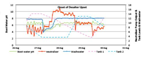
FIGURE 3: IMPACT OF WET CRUDE TANK
